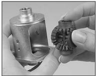
Press-out bevel wheel axle in direction of arrow to mount thrust bearing a.s.o.
