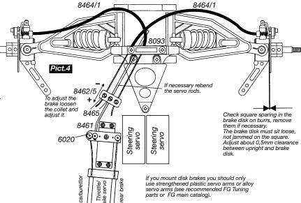
Both brake disks should be turnable with the joystick(transmitter) in neutral position. Both brakes must pursue an equal braking effect on to the disks. If the braking effect is only one-sided, the corresponding bowden cable has to be tightened slightly at the balance 8462/5, therefore loosen the collet 8465. Should the braking effect of both brakes be either too high or too low, loosen the centric collet 8465 at the balance and move the balance 8462/5 either backwards or forwards.
