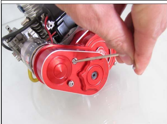
#1: Unscrew the belt wheel cover.
