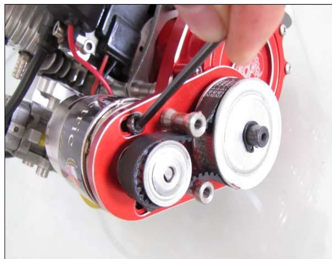
#2: Loosen the motor bolts, and take out the belt.
