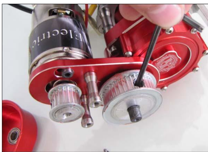
#4: Unscrew the bolt from the main belt wheel.
