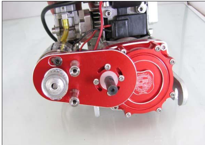
#6: Now you can adjust the motor position by rotating the plate. When positioned as required, tighten the 4 bolts and re-install everything.
